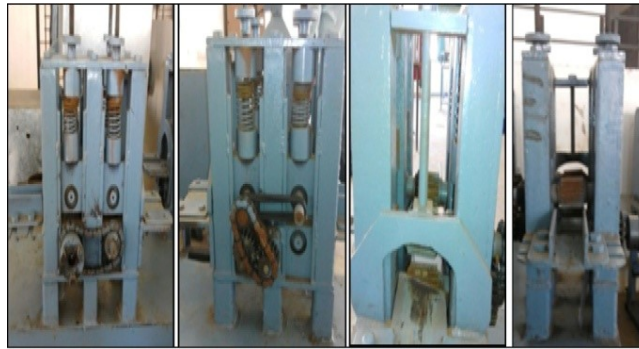
Figure 4: Different views of bamboo sliver cutting unit.
