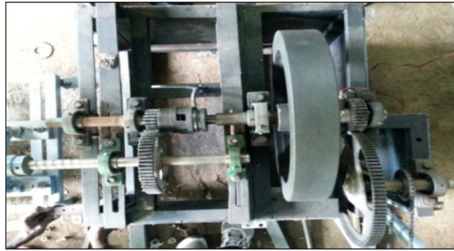
Figure 3: Mechanical power transmission unit.
